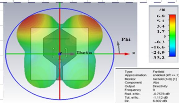
Fig. 13. The 3-dimensional (directivity) radiation pattern
